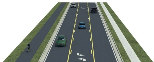
Figure ES-3: Conceptual Three-Lane Typical Section With Shared-Use Path and Sidewalk
