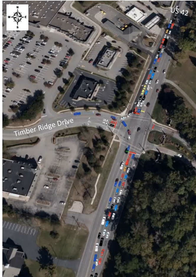
Figure 33. VISSIM 2045 No-Build Typical PM Peak Queue
