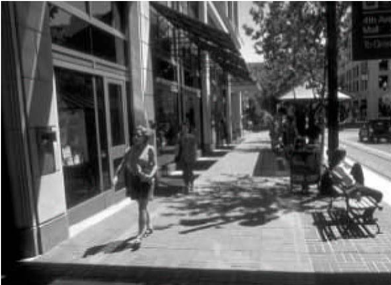
This is a good example of a street furniture zone along the sidewalk on Portland, Oregon's light-rail transit line.
