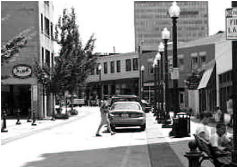
Motorists, bicyclists, and pedestrians share the space on this woonerf or "living street" in Asheville, North Carolina.
