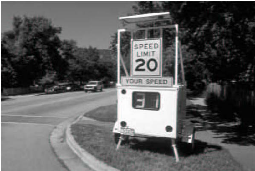
Speed-monitoring trailers let motorists know the speed limit and the speed they are traveling.
