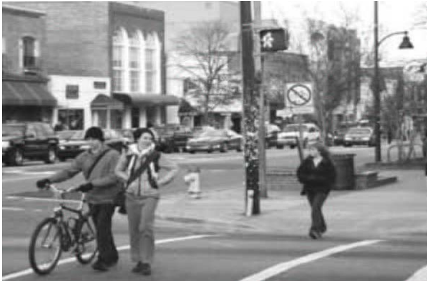
Pedestrian signals should always be clearly visible to the pedestrian while in the crosswalk and waiting on the far side of the street.
