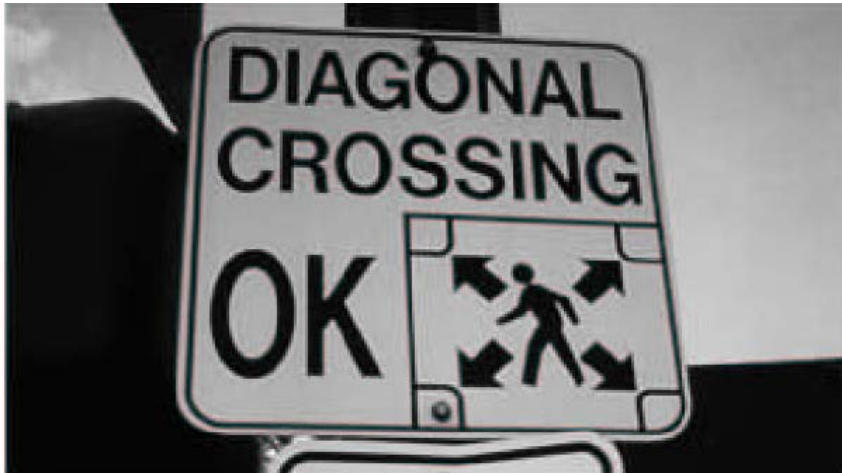
The pedestrian has a dedicated walk phase at this intersection of a busy street and a trail crossing.
