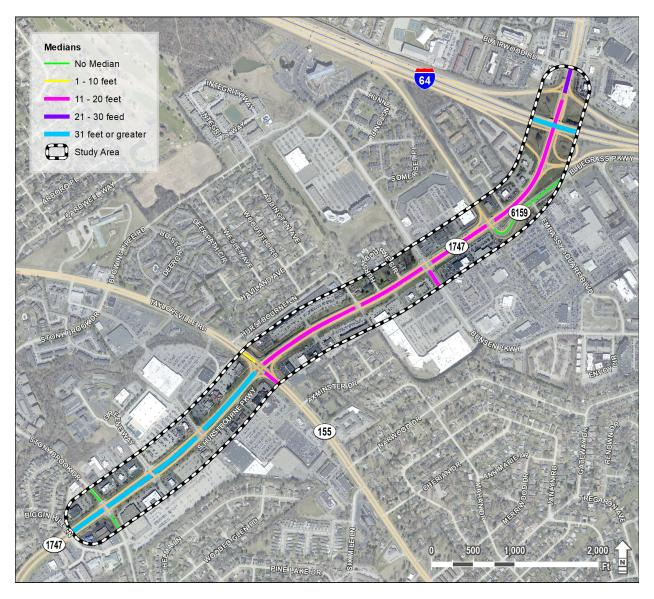
Figure 7: Median Widths along Study Corridor
