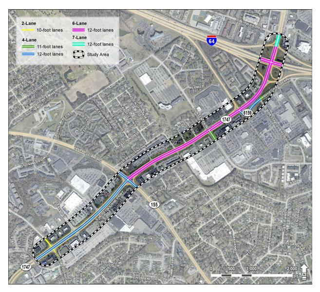
Figure 4: Lane Widths along Study Corridor
