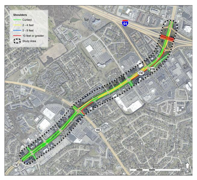
Figure 5: Shoulder Widths along Study Corridor
