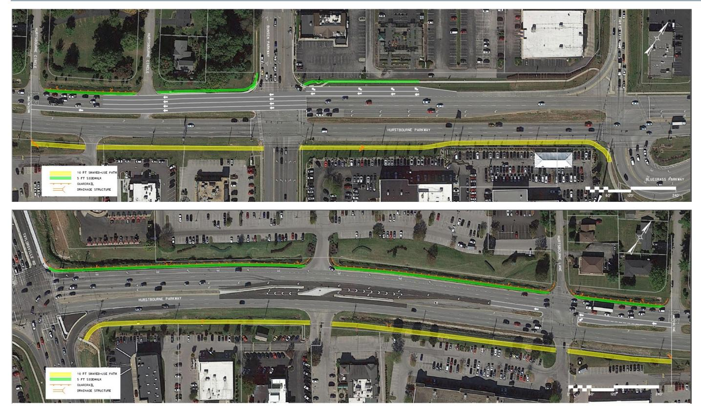
Figure 37: Concept Sketch of Southbound Thru Lane with Pedestrian Facilities
