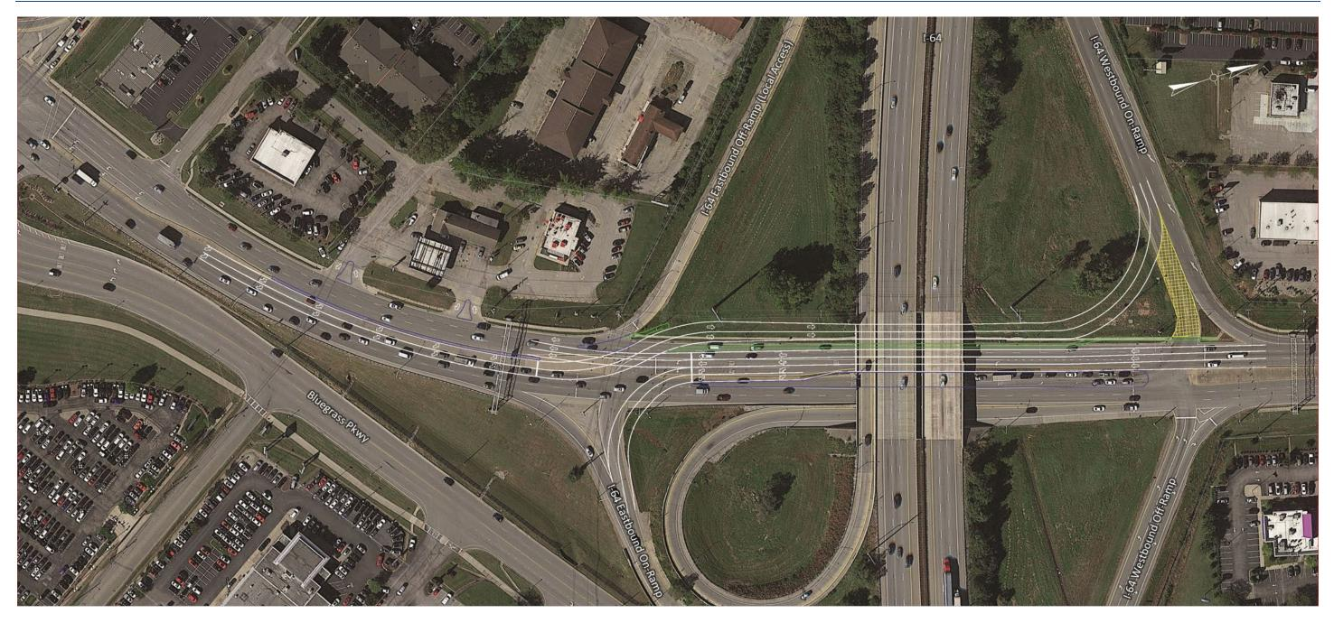
Figure ES - 5: Spot E Concept Sketch of Displaced Lefts
