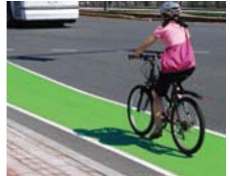
Example of Epoxy Bike Coating on Asphalt
