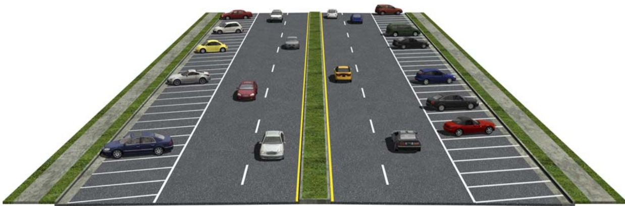
Figure 4-7: Four-Lane, Two-Way Street with Diagonal Parking
