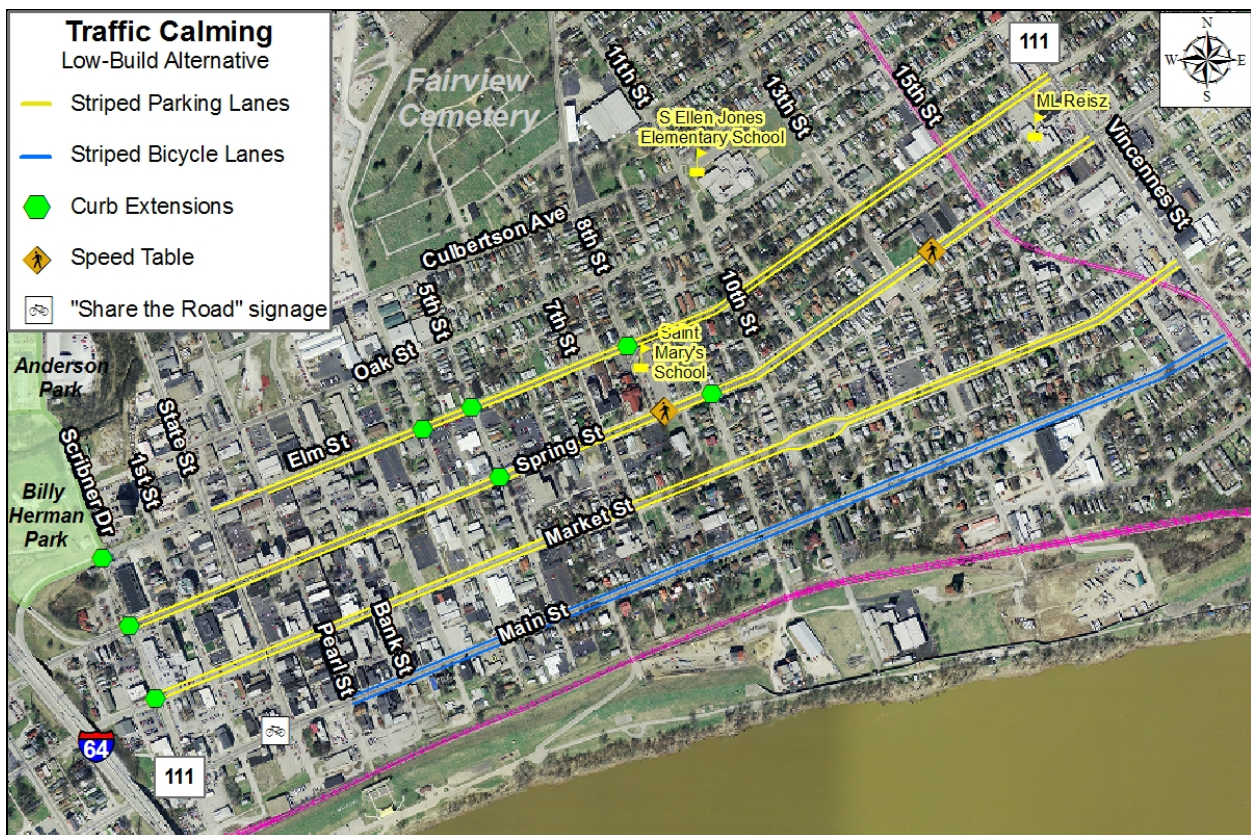
Figure 4-1: Low-Build Traffic Calming Alternative
