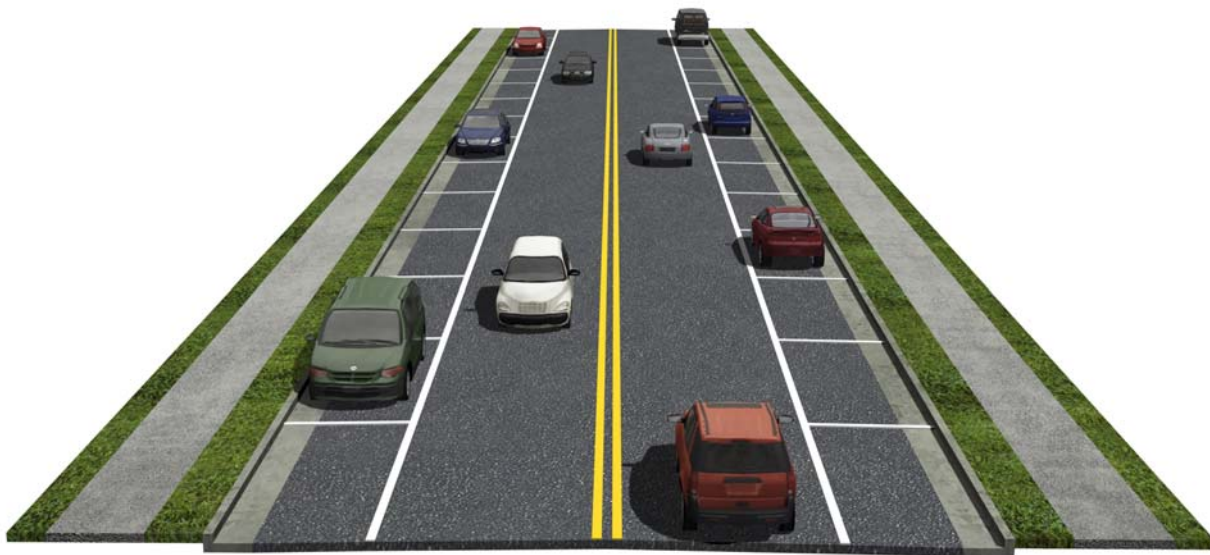
Figure 4-6: Two-Lane, Two-Way Street with Striped Parallel Parking
