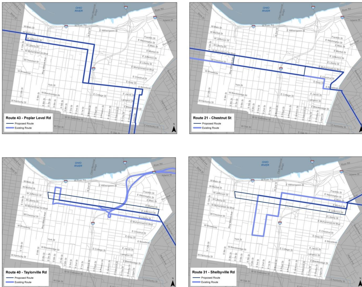
Figure 3.3-10: Proposed Downtown Route Adjustments (Using the Proposed Jefferson and Market Bus Lanes)
