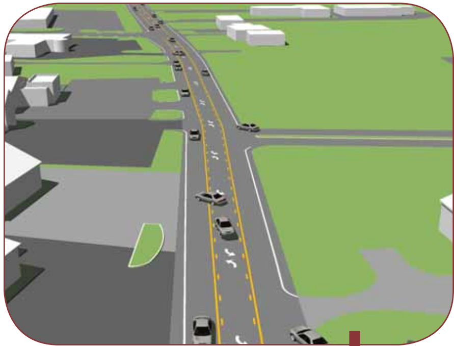
Short-term re-striping in Character Zone 2 Credit: HWC Engineering
