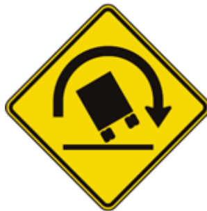
Figure 36. Recommended Supplemental Warning Signage for Ramp 8
